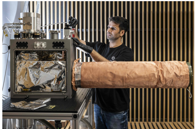
FIG. 8. Our first cryostat housing a cooled pickup coil. It comprises a metallic 4 K stage (on the left) hosting the SQUID sensor, and a vacuum-sealed G10 enclosure at 50 K housing the pickup coil (copper-mesh coated sleeve on the right). This cryostat can accommodate an 80 mm diameter room-temperature sample for some phantom tests.
