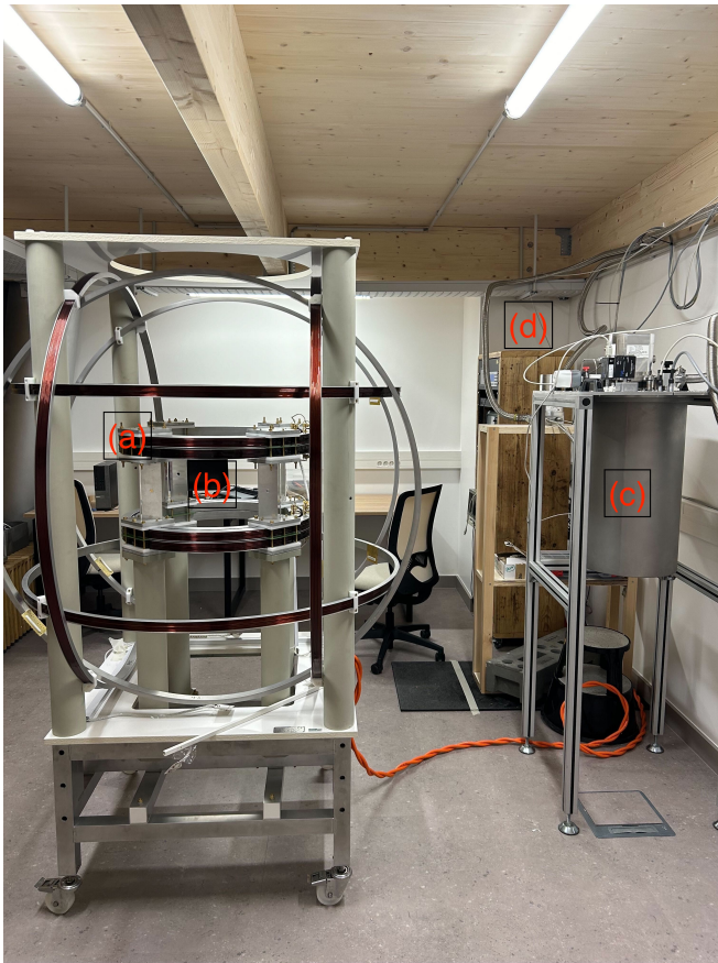
FIG. 7. The Atlantic 10 mT prototype. Like Pacific, the B_0 field is generated by a 40 A current, here through a smaller copper solenoid (a). The sample is placed between the gradient plates and main coil (b). The MRI signal is picked up by a room-temperature copper coil around the sample and sent inside the cryostat (c) where it is amplified by a low- T_c SQUID (SQ2600, STAR Cryoelectronics). In this case, the cryostat is open, revealing the gold-plated structure that cools the SQUID. This room-temperature pickup coil can also be cooled with the custom cryostat described in Fig. 8. The signal is then read out by room-temperature electronics in the rack (d).
